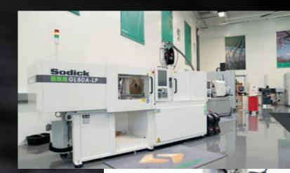
Sodick developed the revolutionary V-LINE® technology to deliver high-precision moulding. By separating the plasticisation and injection processes, a stable molten state is achieved with highly accurate repeatable mould filling.
